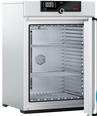
The indispensable safety feature for this hot air steriliser: Setpoint Wait. This means that the programme for sterilisation only starts when the set temperature has been reached. This feature can also be used with freely positionable Pt100 temperature sensors. Here the sterilisation time only begins when the set temperature has been reached at all measurement points, and reliable sterilisation is guaranteed at all times.
