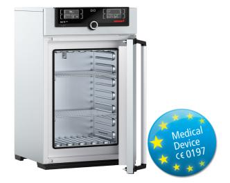
The indispensable safety feature for this hot air steriliser: Setpoint Wait. This means that the programme for sterilisation only starts when the set temperature has been reached. This feature can also be used with freely positionable Pt100 temperature sensors. Here the sterilisation time only begins when the set temperature has been reached at all measurement points, and reliable sterilisation is guaranteed at all times.
